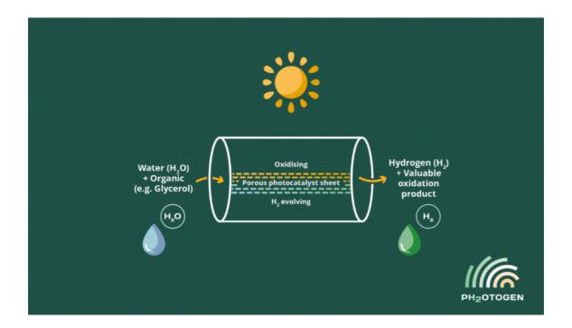
The PH2OTOGEN project has developed an innovative demonstrator that utilises sunlight to produce green hydrogen while oxidising low-value organic molecules, such as glycerol, into valuable chemicals.
